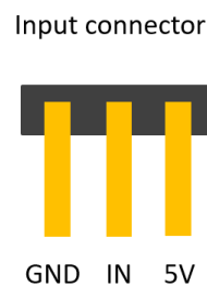
Figure 7.2: SK 0 input connector
