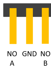
Figure 7.5: SK 0 output connector
