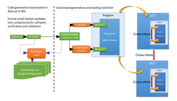
Safety is based on a software library (covered by the SIL4 certificate) on top of which the final user can develop its custom application. The only constraint consists of calling periodically a set of primitives to perform vital health tests, otherwise, the system will fall back into safe state mode.
