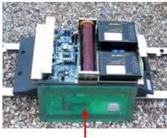
■ Inside view with the patented frequency frame (green plate)
