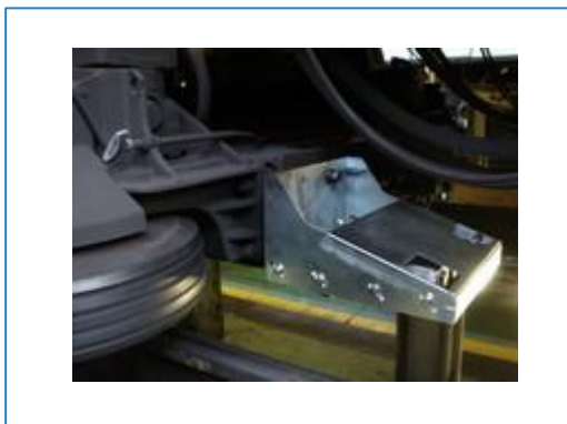
■ Onboard DOF1 loop antenna prototype fixed onto the bogie
