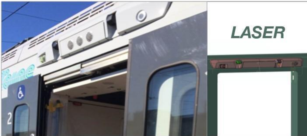
■ Lasers mounted next to the door
