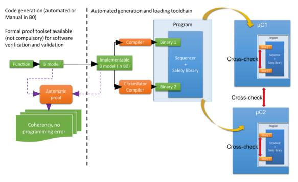
Safety is based on a software library (covered by the SIL4 certificate) on top of which the final user can develop its custom application. The only constraint consists of calling periodically a set of primitives to perform vital health tests, otherwise, the system will fall back into safe state mode.
