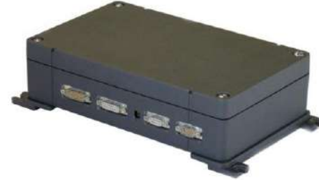
Onboard unit (sensor and train doors interface)
