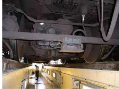
Sensor mounted under the train (bogie)
